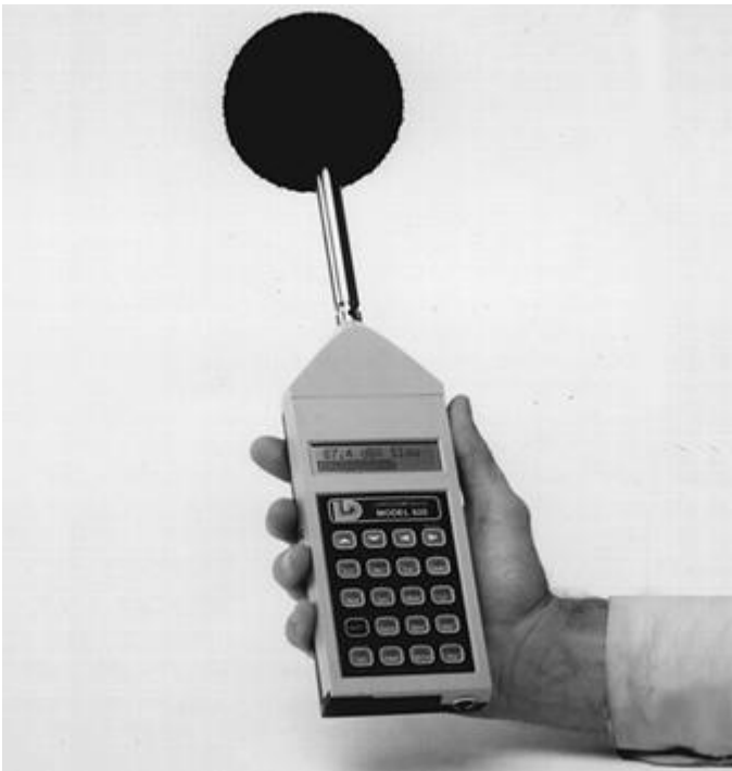
Figure 2. Sound level meter with wind screen. Courtesy of Larson Davis
