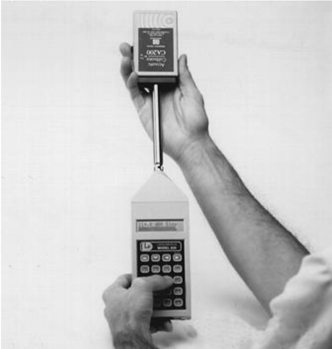
Figure 2. Sound level meter with wind screen. Courtesy of Larson Davis
